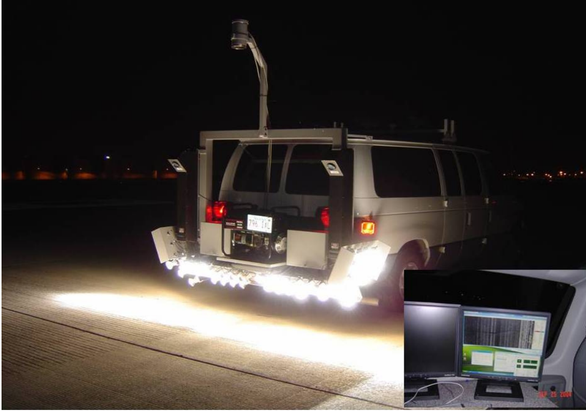
Figure 2 – Automated Digital Video Mapping Van and Recording Equipment
