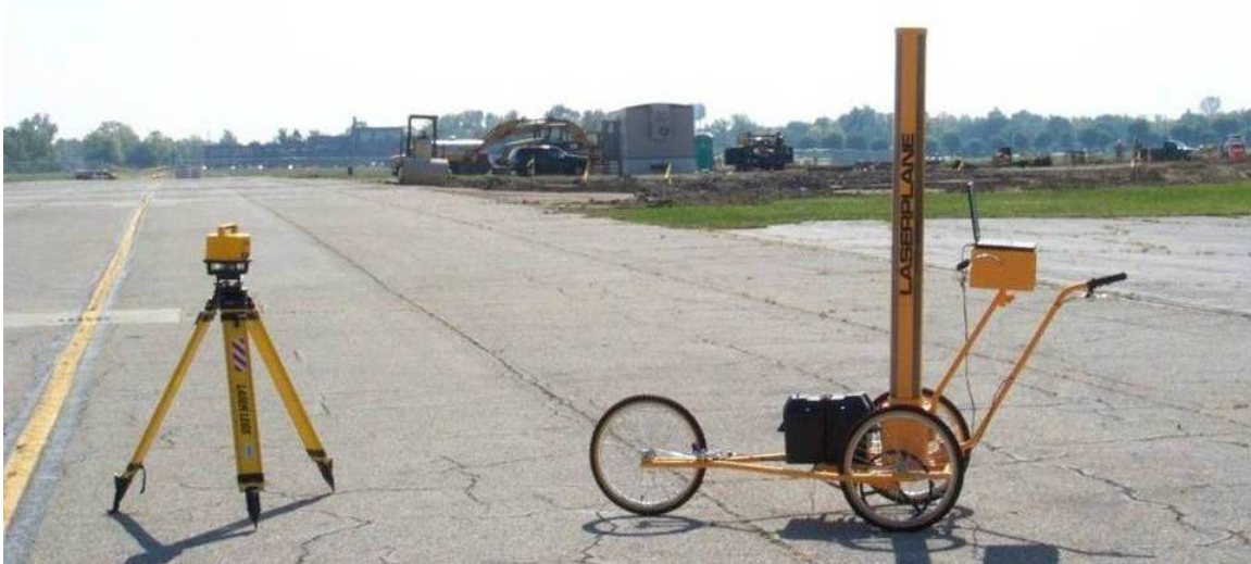
Figure 6 – Laser Source (left) and Cart System (right) for Profile Measurements
