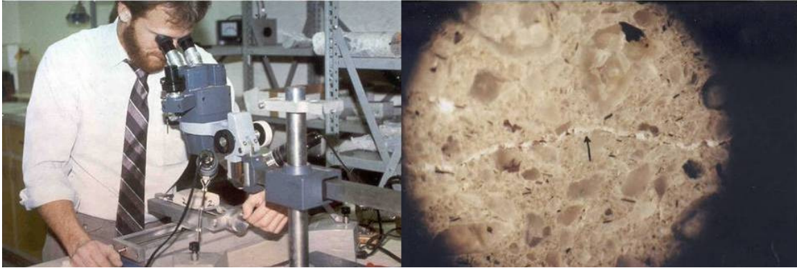
Figure 10 – Petrographic Examination of Concrete Core with Binocular Microscope
