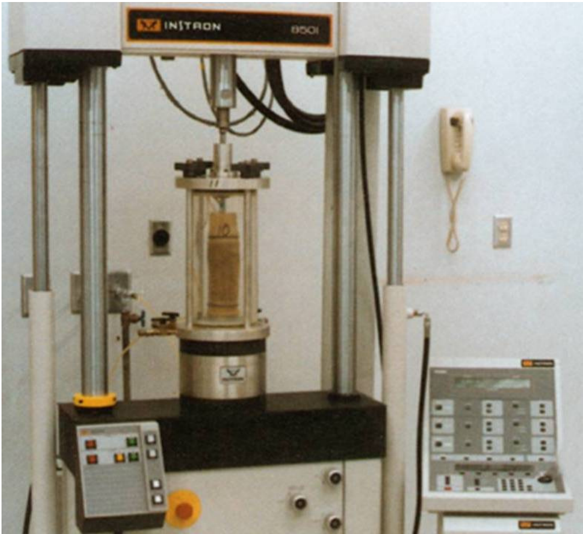
Figure 9 – Resilient Modulus Test Equipment for Subgrade Soil Characterization
